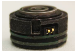
Figure 8c: Align opposite the key in the Module housing
