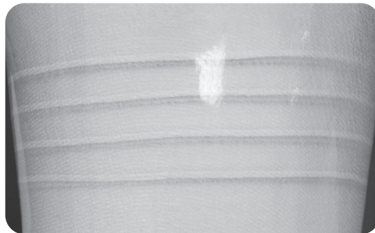
INCORRECT: All four fins are not contacting the socket.
