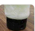
Apply the carbon tape around the 4-Hole Adapter.
