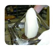
Tape off the hole in the 4-Hole Adapter. Tape off any holes in the socket.
