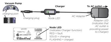
Charge the Vacuum Pump in a well-ventilated area between 5 °C (41 °F) and 32 °C (90 °F). Charging outside of this range may damage your Vacuum Pump. It may also result in prolonged or incomplete charging.
