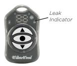
If the pump detects a leak, the red **Leak Indicator** will light up. Also, the system will enter **Standby State**.
