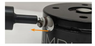
• Use the extraction tool to remove the second check valve in the same way as you removed the first one.
