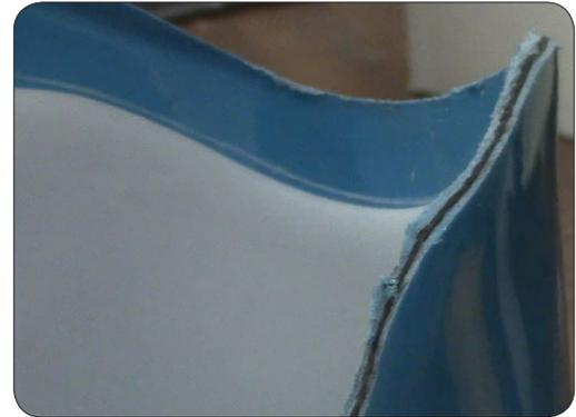
13. Sand and polish the laminated socket edges so that the finished laminated socket is 1/8" (3 mm) higher than the flexible socket everywhere except in the posterior area, where the laminated socket should blend to match the flexible socket.
