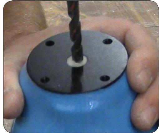
16. Push the poron filter into the hole. Cut it flush with the socket.
