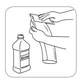
Place a small amount of ethyl or isopropyl alcohol on a soft, clean cloth. Lightly wipe the side of the liner without the logo with the cloth for two minutes.
